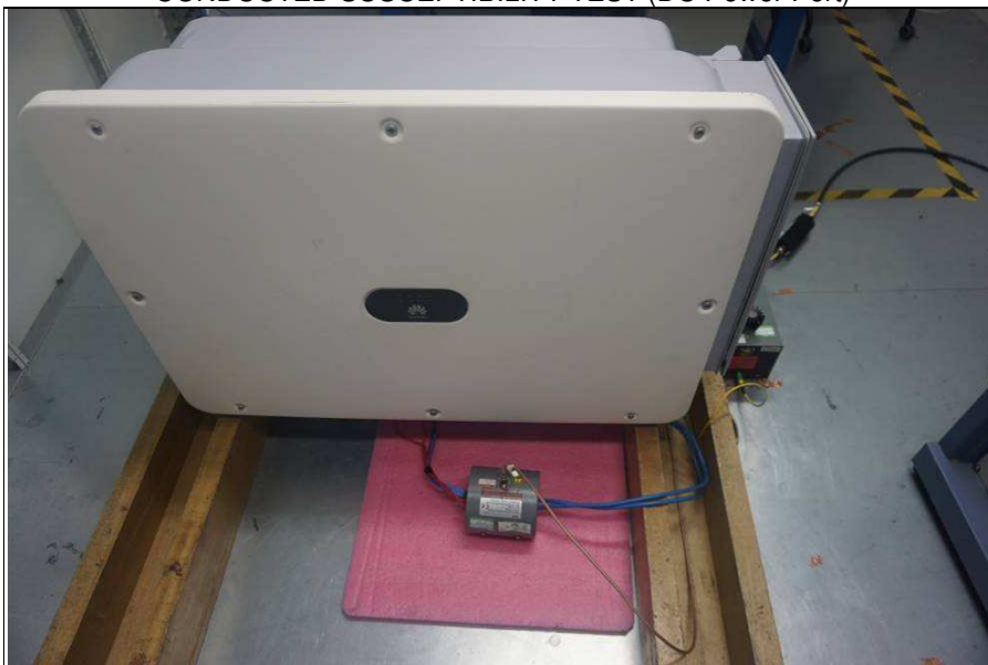
CONDUCTED SUSCEPTIBILITY TEST (DC Power Port)
