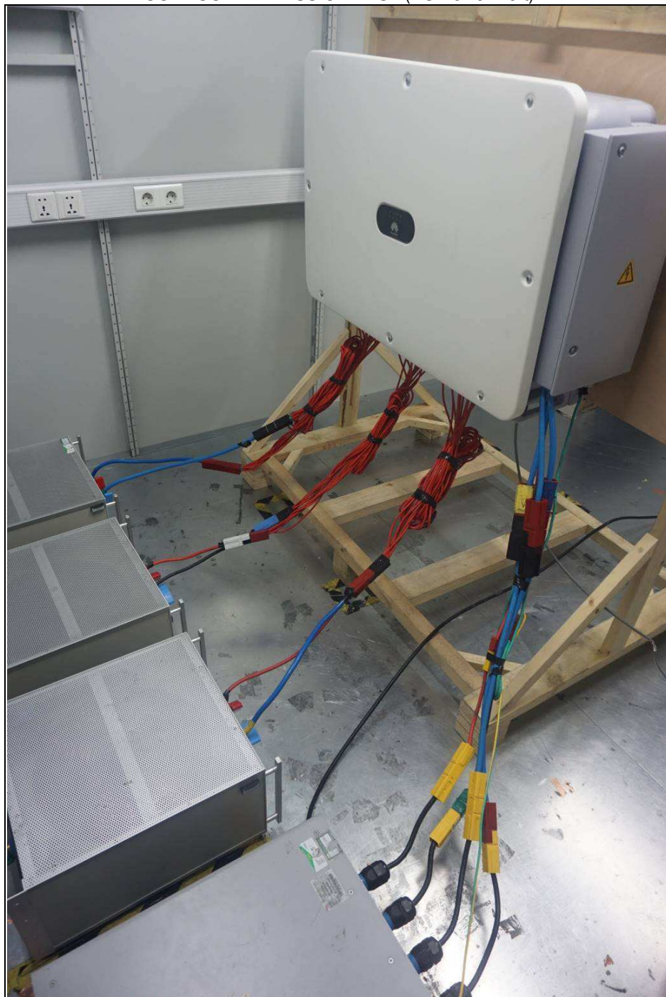
CONDUCTED EMISSION TEST (AC Power Port)
