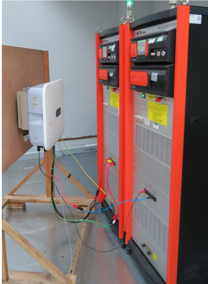
Immunity to surges of DC input & AC output Power Port
